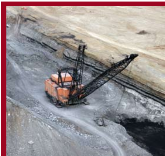
Dragline excavator at a strip mine in northwestern New Mexico, much like those that are being proposed for Alaska. The coal seams are clearly visible. Photo by Dean Cully, http://deancully.zenfolio.com/
